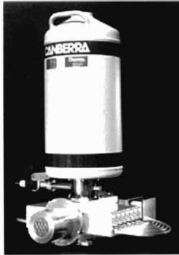
Figure 4.11. Photograph of a multi-element solid-state Germanium detector. This image shows a 13-element detector. A 100 element Ge detector is in use at the Photon Factory synchrotron source in Japan.
