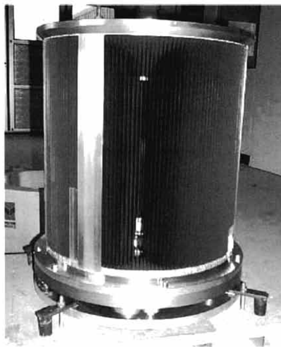
Figure 4.6. Photograph of the radial collimator that is now installed on GEM at ISIS. The vertical vanes are thin and borated.
